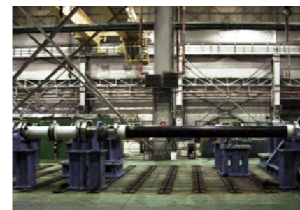
Carbon Fibre Shaft combined with LAMIDISC® coupling.
