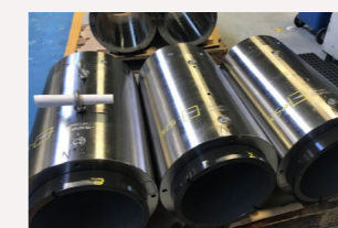
Sleeve type JHC-HF-S (Max Torque 960kNm)
